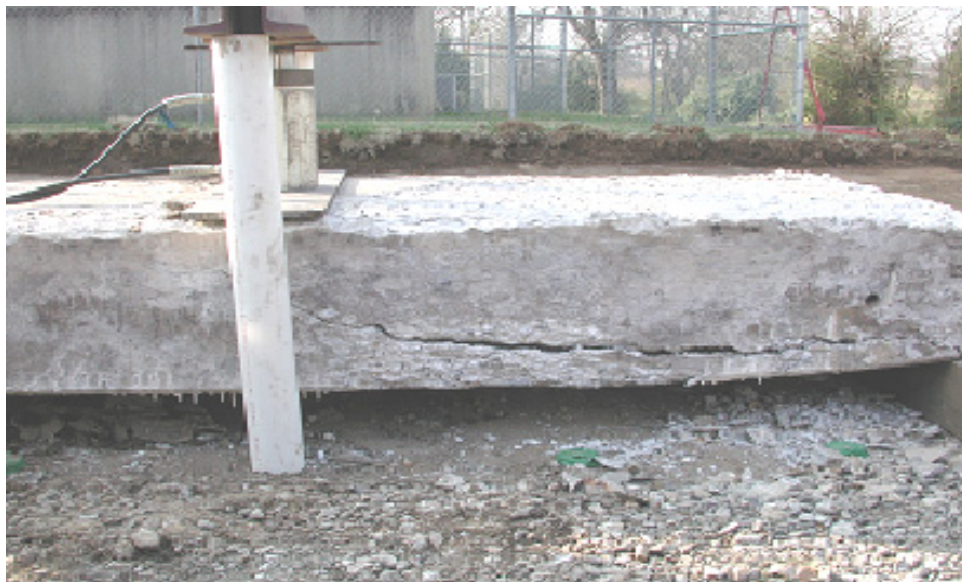
Figure 13: Stalactites on Underside of Panel
