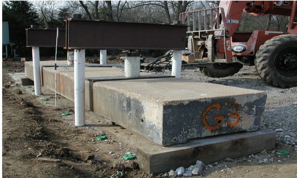
Figure 27: Gentry Beam with No Signs of Distress
